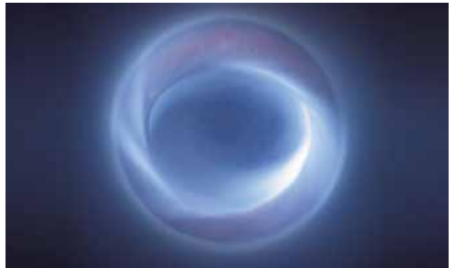
Lean gas flame – stable combustion without any supporting fuel
